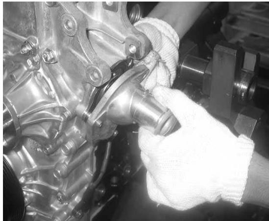
**Gambar 18. Proses Pemasangan Thermostat, Gasket, WTI**
